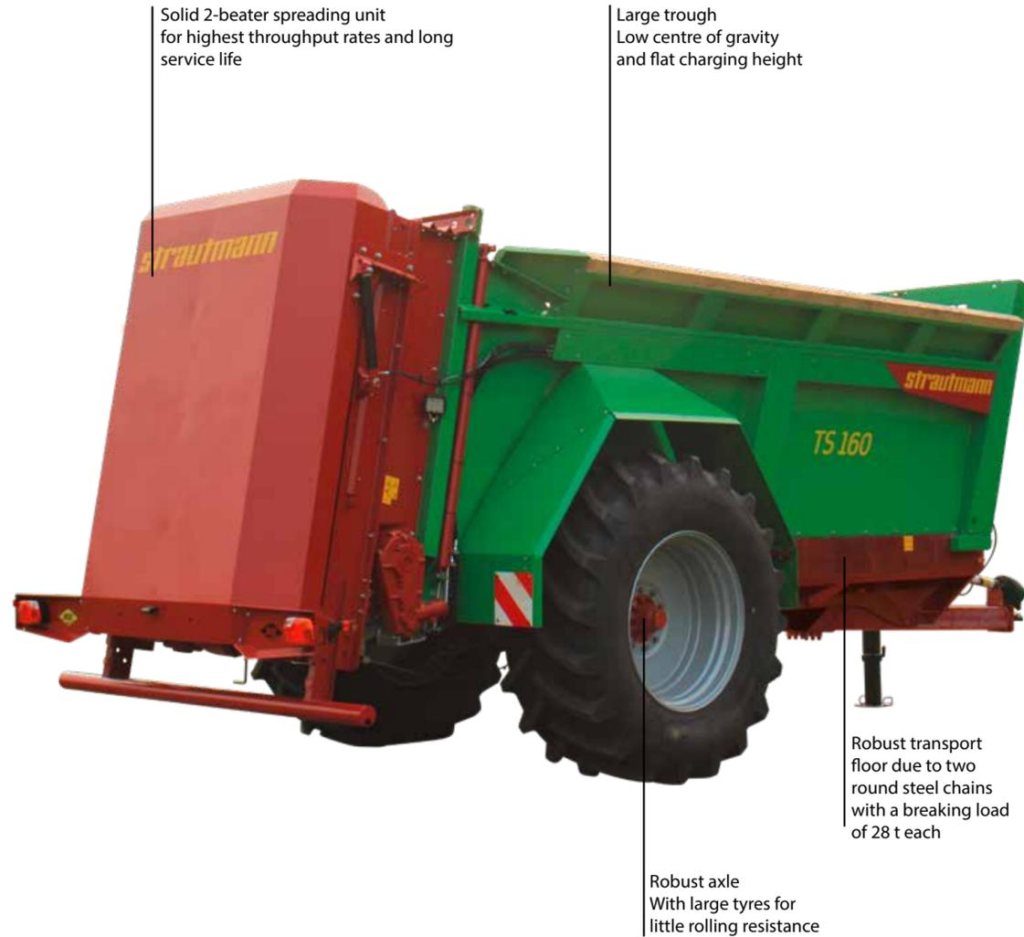
Solid 2-beater spreading unit for highest throughput rates and long service life
