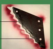
Knife tip <1 mm of residual thickness
