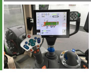
Due to the compatibility of the Strautmann ISOBUS control (ISOBUS AEF certification), most varied terminals can be used for the Strautmann forage wagons. Thus, depending on the tractor type, all machine functions can also be operated via the tractor joystick.
