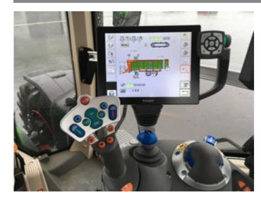
Due to the compatibility of the Strautmann ISOBUS control (ISOBUS AEF certification), most varied terminals can be used for the Strautmann forage wagons. Thus, depending on the tractor type, all machine functions can be operated via the tractor joystick.
