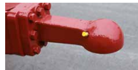
Coupling head linkage K80
