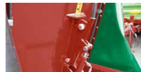
Counter-cutter (hydraulic adjustment)
