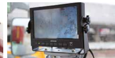
Monitor for rear-view camera
